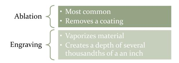
Each marking technique produces different looks on the aluminum, dependent on the type of aluminum being marked. Each technique is also accomplished in a unique way.
